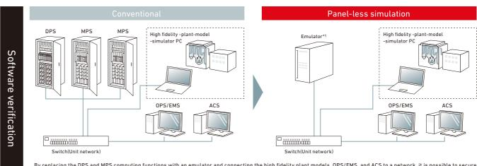
By replacing the DPS and MPS computing functions with an emulator and connecting the high fidelity plant models, OPS/EMS, and ACS to a network, it is possible to secure enough time for verification at the plant even after control panel (hardware) shipping. This makes it possible to reduce the man-hours necessary for on-site system-up verification as well as costs and to speed up the start of operations by customers.
