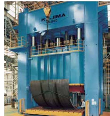
6,000-ton Hydraulic Press
