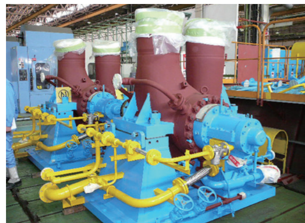
Main Feedwater Pump (MHI)
