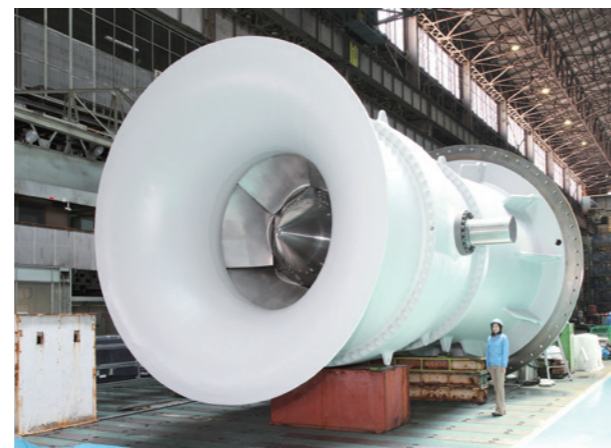
Circulating Water Pump (MHI)
