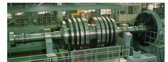
Mono-block Rotor (for thermal plant)
