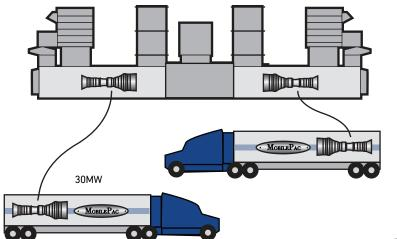
One or both gas generators and power turbines are removed "as is" from your stationary gas turbine package and installed into the MOBILEPAC® trailers, giving you one or two blocks of mobile power.
