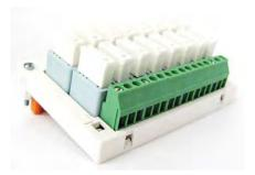
\*Wire holding structure : Screw type
