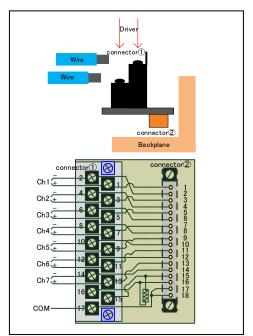
\*1 screw-up type: It is a terminal block of screw dropout prevention function type.
