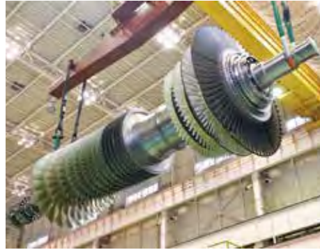
M501 JAC Gas Turbine Rotor
