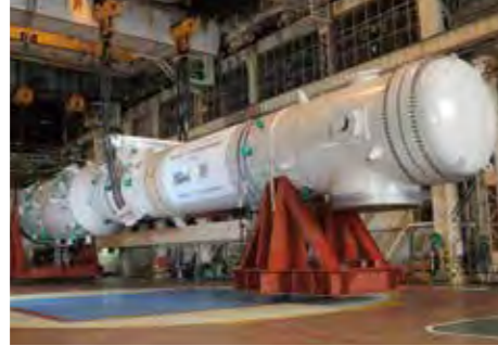
Integrated Coal Gasification Combined Cycle Gasifier
