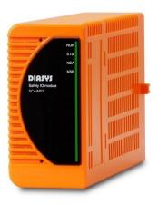
\*Number of input channels . 8 ch (Channel individual insulation)
