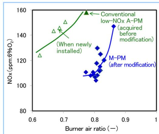
**Figure 8 Comparison of H5 unit characteristics for NOx generation**
