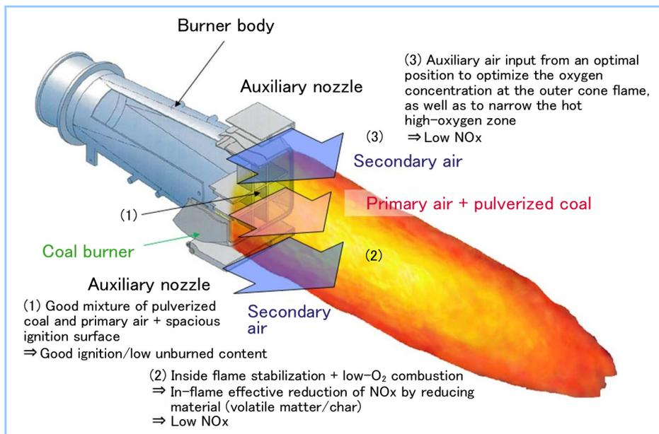
**Figure 2 M-PM burner concept**
