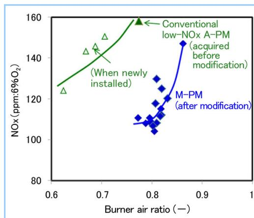
**Figure 8 Comparison of H5 unit characteristics for NO<sub>x</sub> generation**
