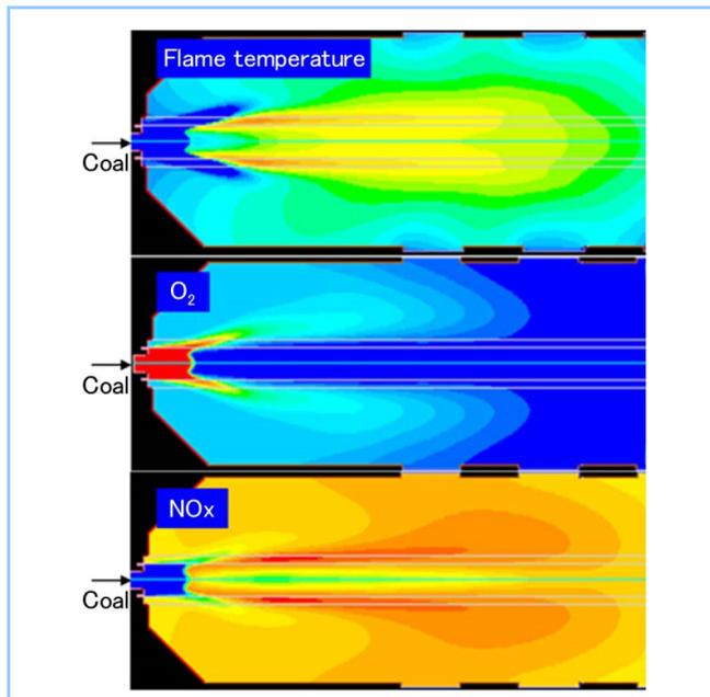
**Figure 1 Analytical results of conventional low-NO<sub>x</sub> A-PM burner**
