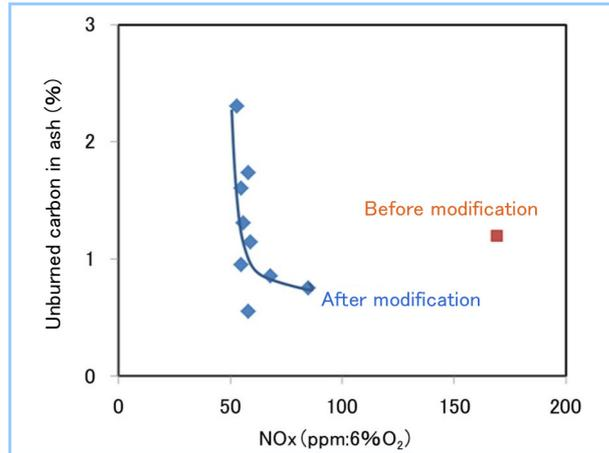
**Figure 6 Comparison of Z2 unit performance before/after modification**
