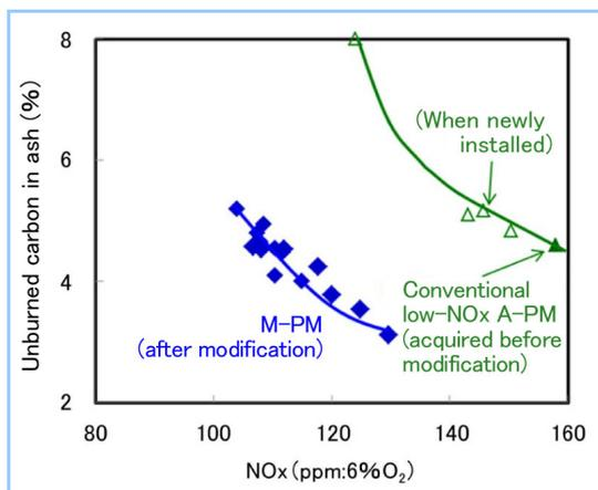
**Figure 7 Comparison of H5 unit performance before/after modification**
