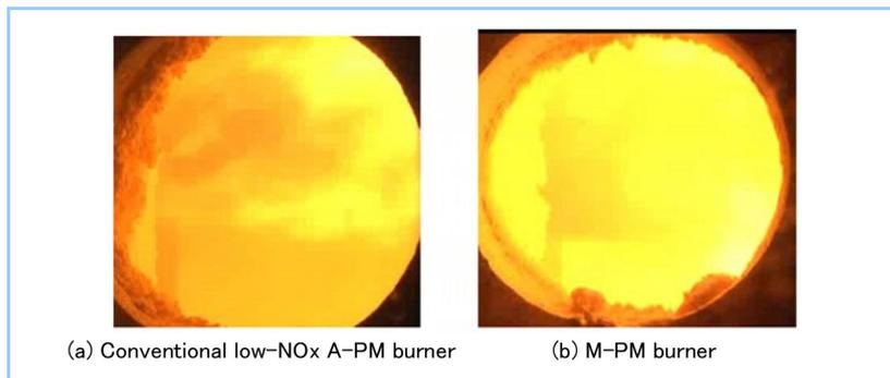
**Figure 3** State of combustion in 4-t/h single-burner test furnace
