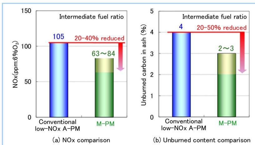
**Figure 4** NO<sub>x</sub>/unburned content comparison for 4-t/h single-burner test furnace
