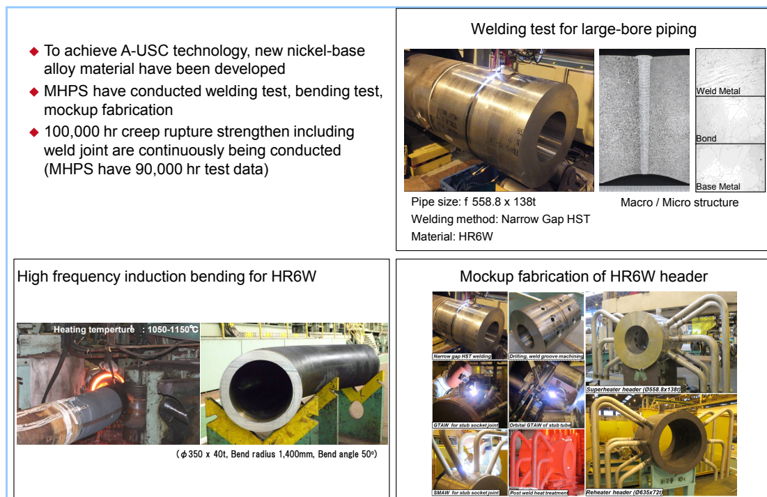
Figure 9 Candidate material development tests for A-USC boiler
