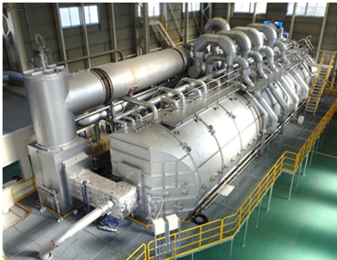
Figure 11 Exterior view of the 4 t/h combustion test facility
