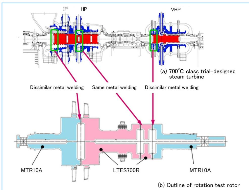
**Figure 11 Rotor design concept for rotation test**
