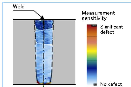
Figure 14 Nondestructive inspection results of weld
