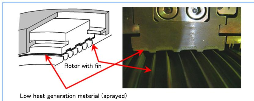
**Figure 6** Abradable ACC seal
