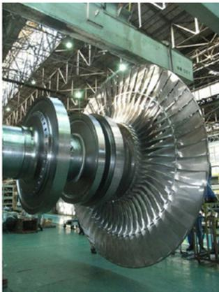
Figure 1 External view of 50-inch blade for 3600 rpm
