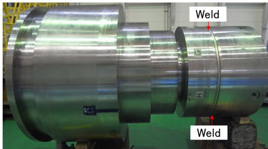
Figure 13 LTES700R welded rotor
