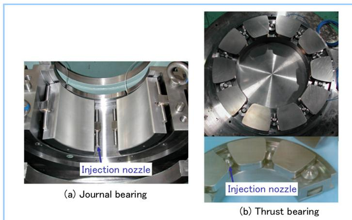
**Figure 8** Direct lubrication journal and thrust bearings
