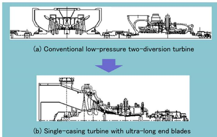
**Figure 4** Application example of large GTCC steam turbine
