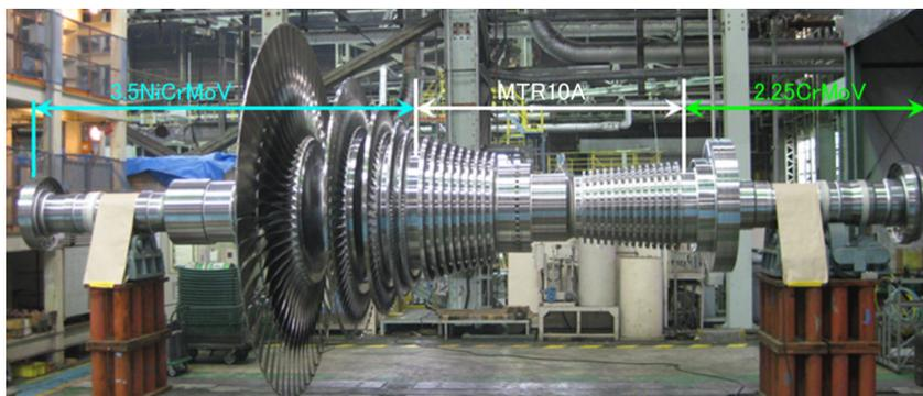
**Figure 9** SRT50 welded rotor
