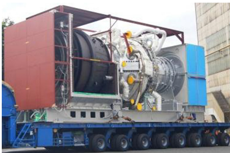
Figure 12 H-100 gas turbine, to be supplied to the IGCC demonstration facility (OCG Project)
