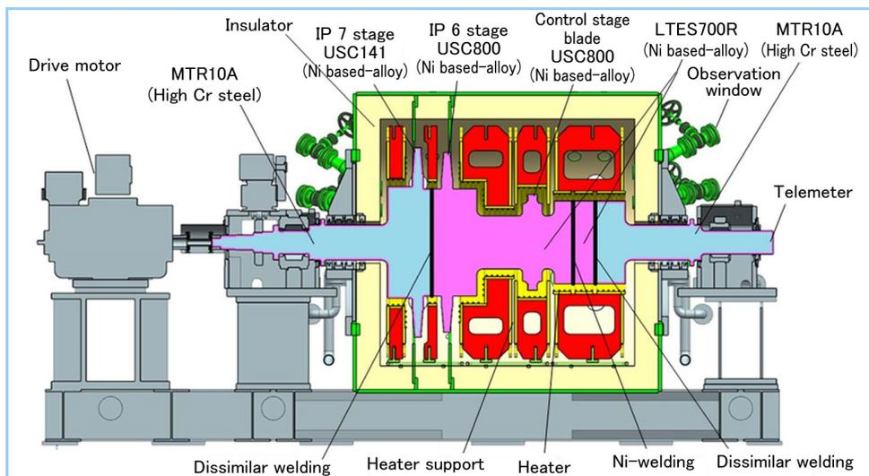
**Figure 7** Rotation test rotor and design plan structure
