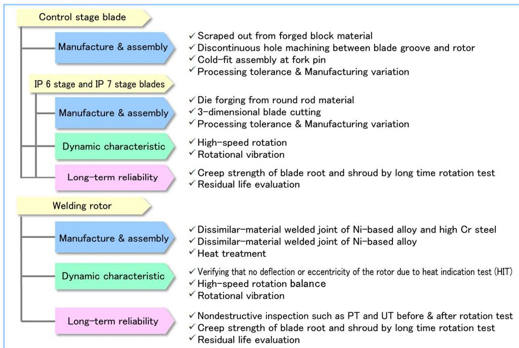
Figure 5 Rotation test verification items
