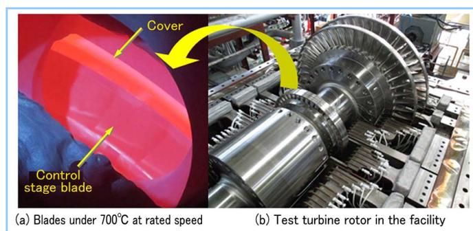
**Figure 8** Test turbine rotor and control stage blade
