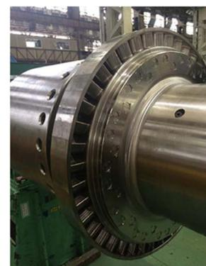
**Figure 4** Manufacturing example of control stage blade
