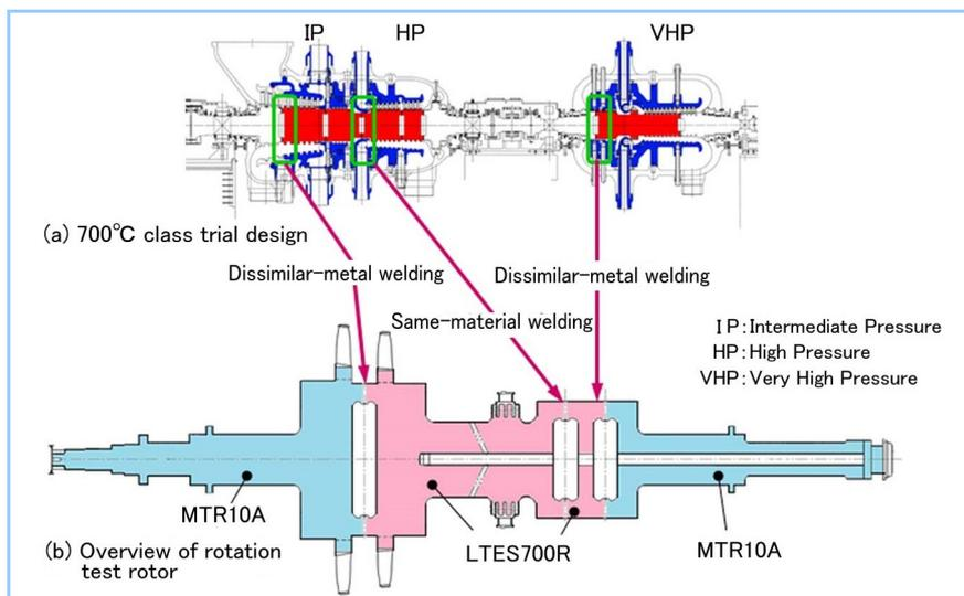
Figure 6 Rotor design concept for rotation test
