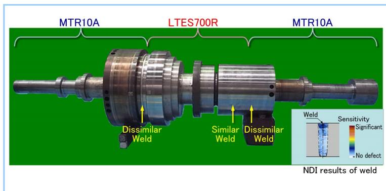
**Figure 3** Example of welded rotor application and nondestructive inspection
