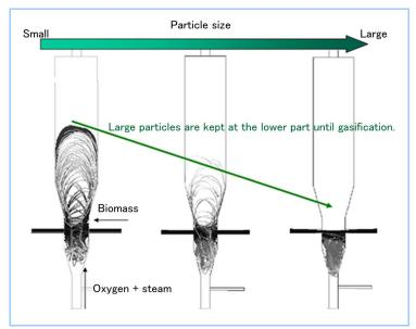
Figure 2 Biomass particle behavior in a gasifier
