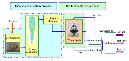
Figure 1 Bio jet fuel production process
