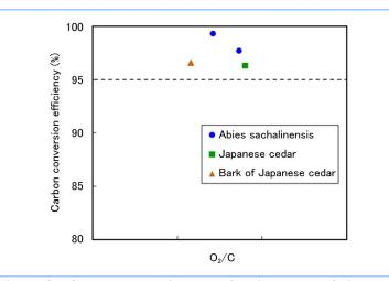
Figure 3 Carbon conversion rate of various types of biomass
