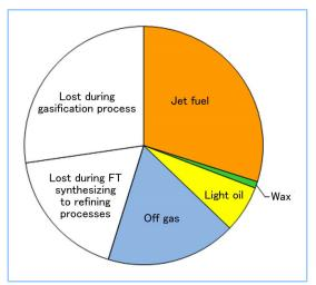
Figure 6 Bio jet fuel production process Heat balance
