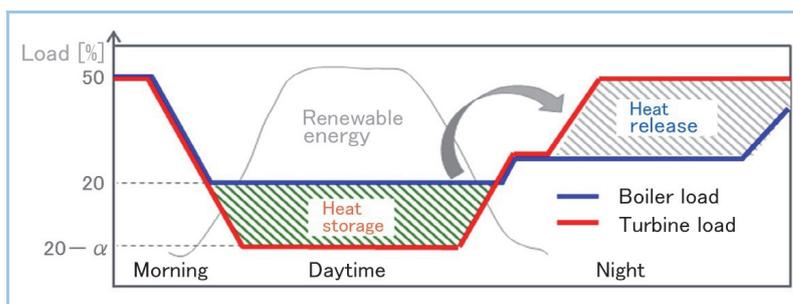
Figure 13 Heat storage resulting from difference between boiler load and turbine load and converting it into power
