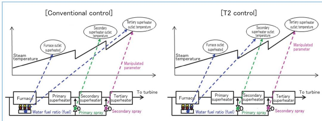
**Figure 5 Comparison of conventional control and T2 control (manipulated parameters of each outlet temperature)**
