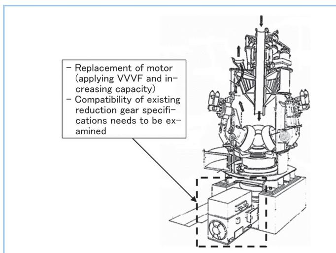
**Figure 15** Major mill modifications accompanying reexamination of mill band operation
