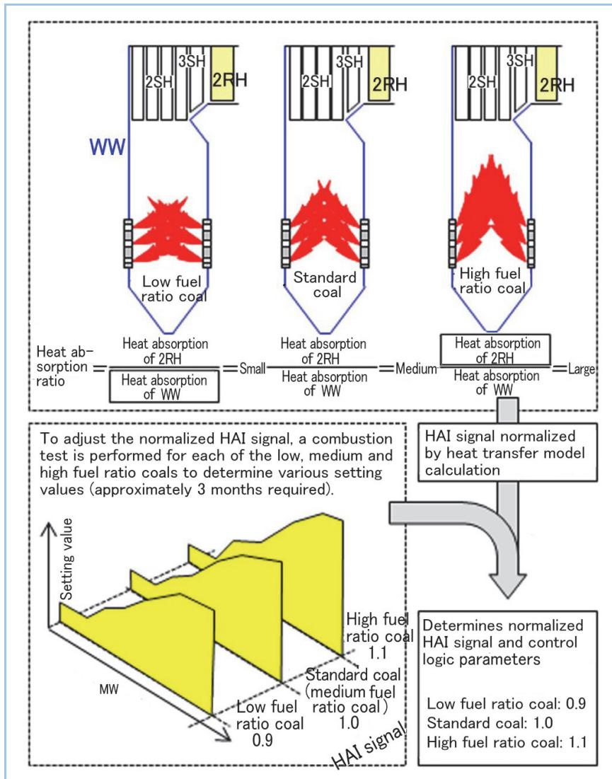
Figure 8 Concept of multi-coal type control
