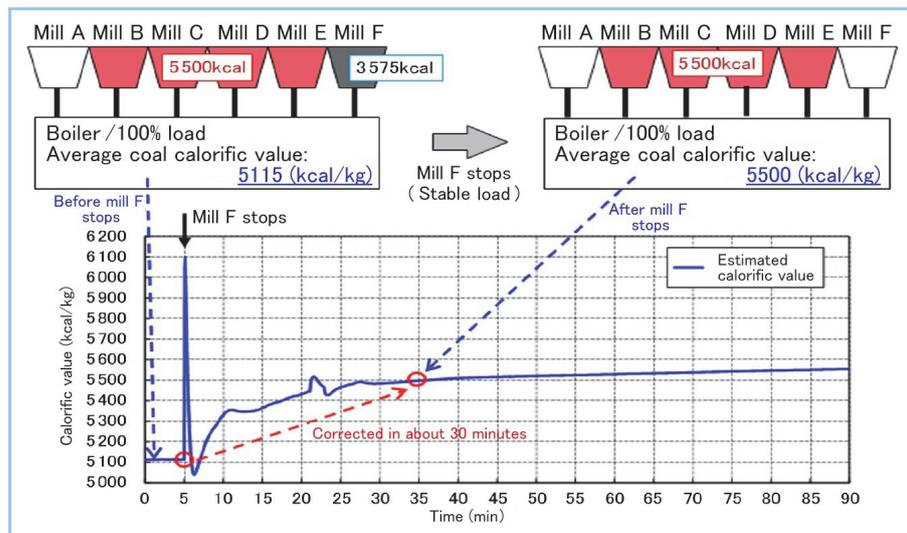
Figure 9 Improvement of calorific value fluctuation correction method
