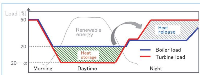
Figure 13 Heat storage resulting from difference between boiler load and turbine load and converting it into power
