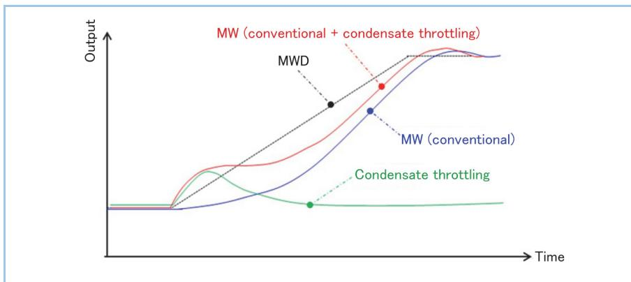
**Figure 7 Effect of utilization of condensate throttling**
