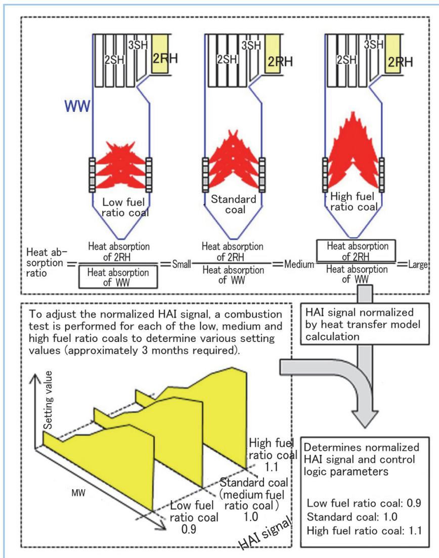
Figure 8 Concept of multi-coal type control
