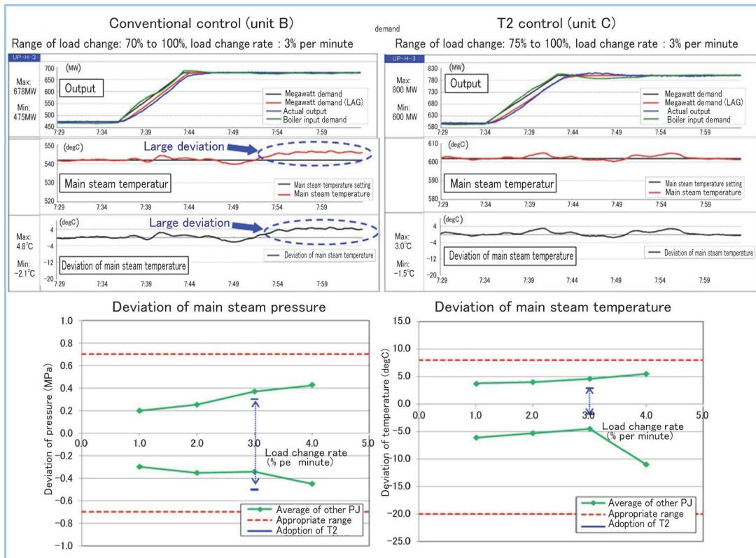
**Figure 6 Comparison of actual operating data between conventional control and T2 control**
