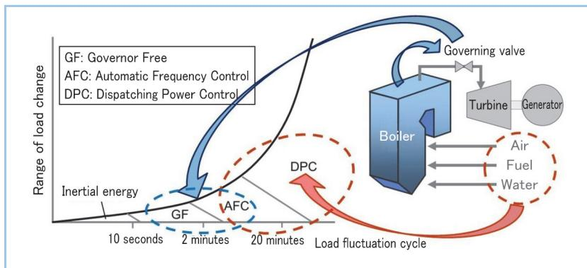
**Figure 2 Control capability with regard to load fluctuation cycle and range of load change**
