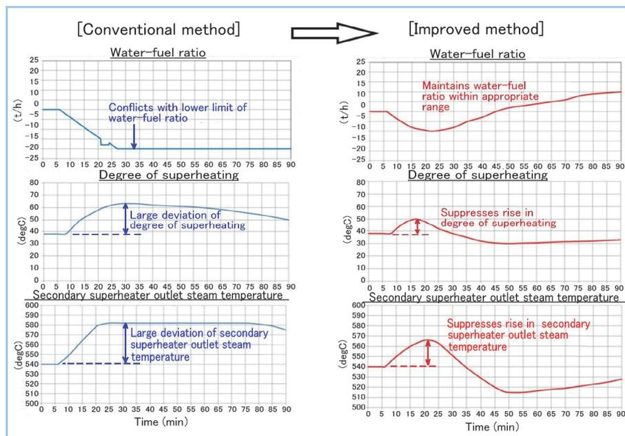
Figure 10 Steam temperature control using calorific value fluctuation correction
