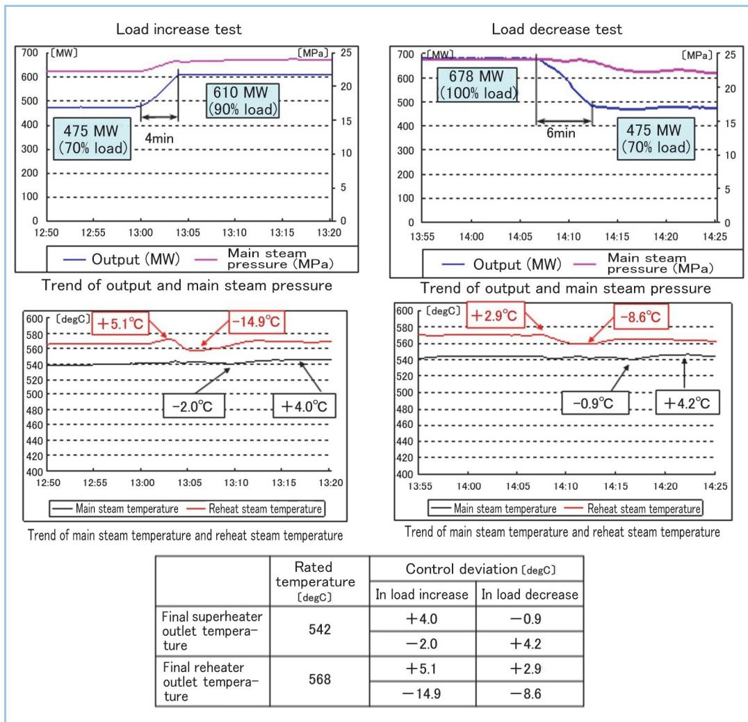
**Figure 4** Results of response to high-speed load change
