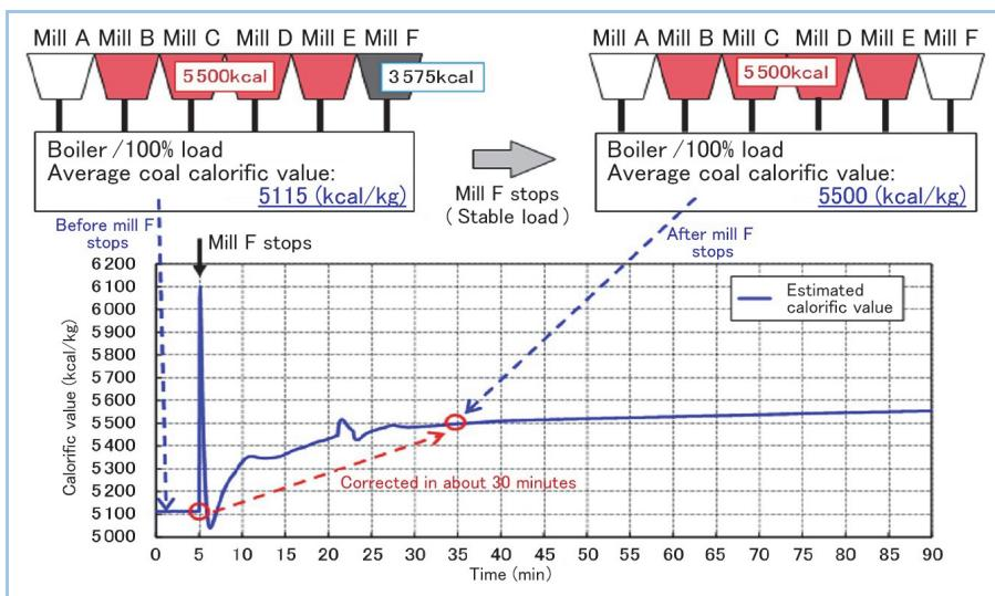
**Figure 9 Improvement of calorific value fluctuation correction method**
