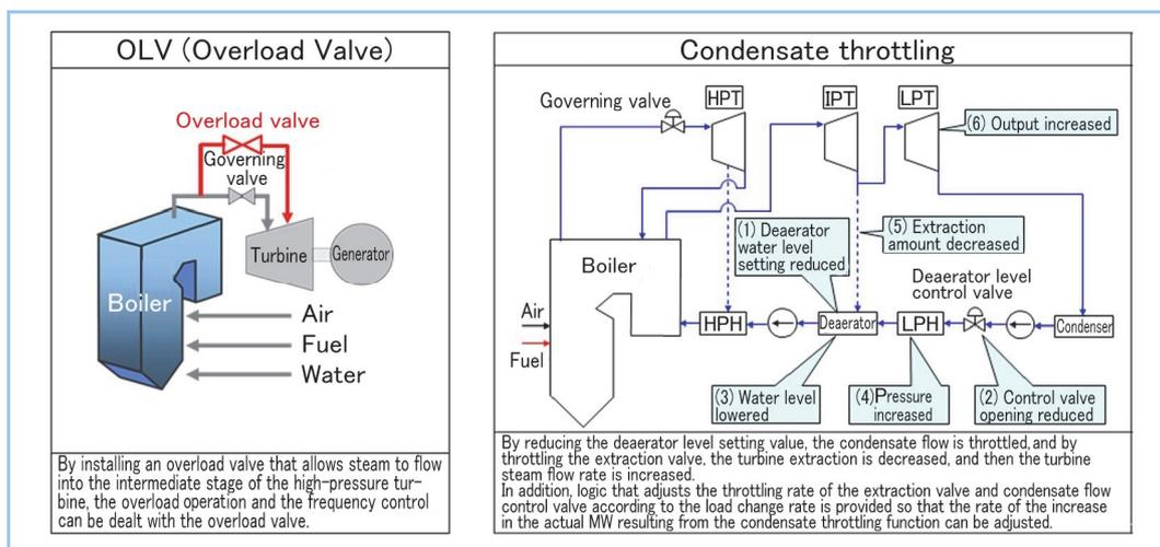
**Figure 3** Load increasing method of high-efficiency boiler
