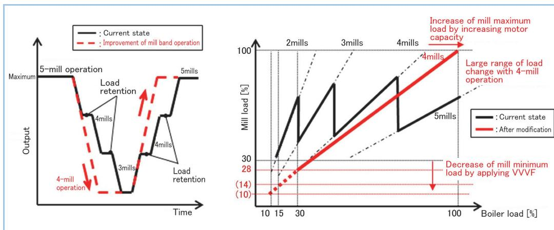
**Figure 14 Improvement of operability by reexamination of mill band operation**
