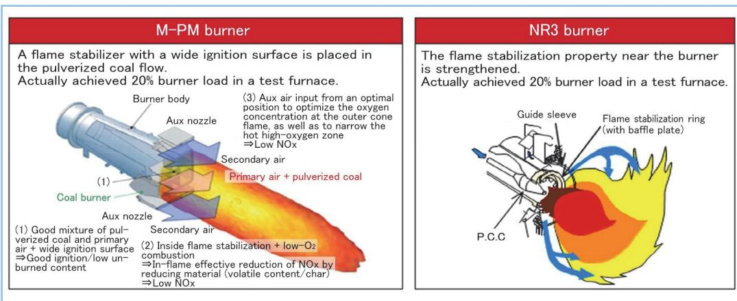
Figure 11 Our latest coal-fired burners
