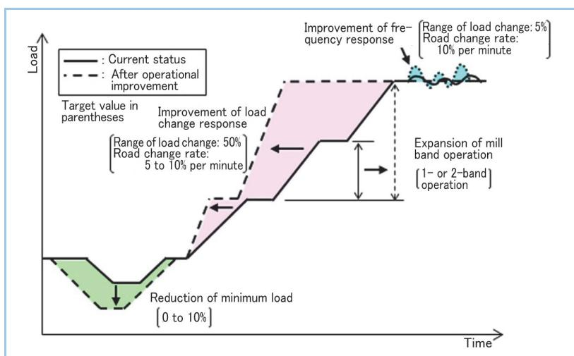
**Figure 1** Latest boiler load adjustment capability improvement menu
