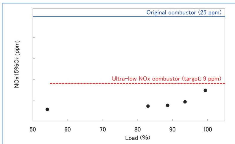
**Figure 3 Trial operation result of Datran Power Plant**
