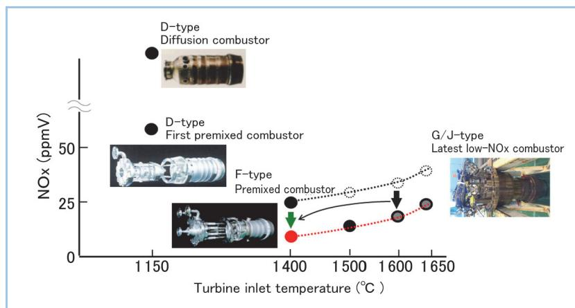
**Figure 1 Transition of relationship between increase of T1T and development of combustor**
