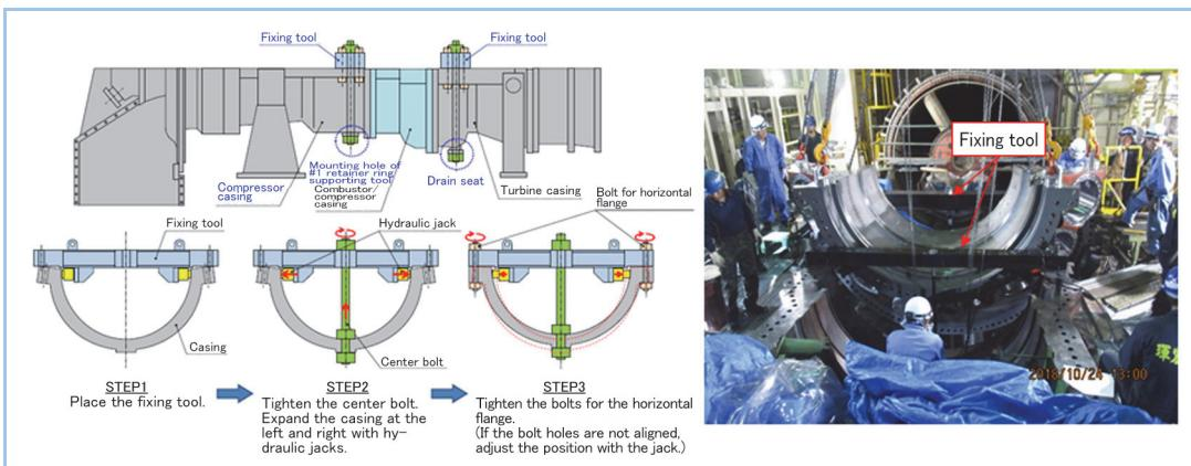
**Figure 5 Fixing tool for correcting egg-shaped deformation of existing casing**
