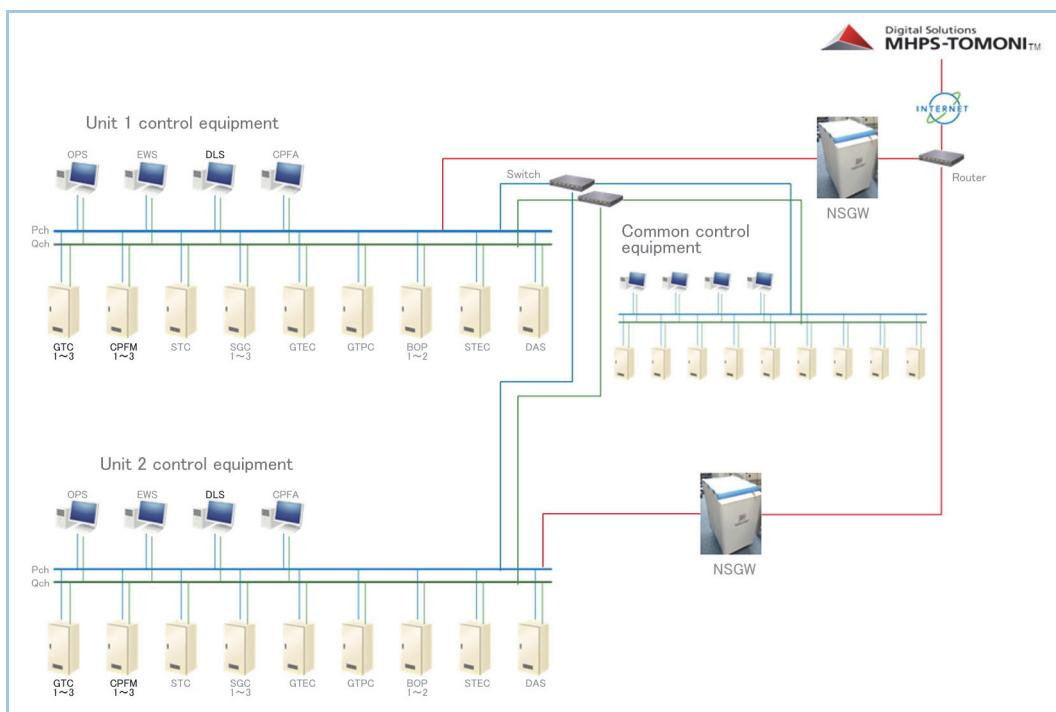
**Figure 6** Remote monitoring system configuration diagram (Datan Power Plant)
