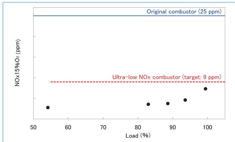
**Figure 3** Trial operation result of Datan Power Plant
