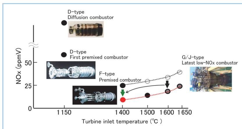
Figure 1 Transition of relationship between increase of TIT and development of combustor
