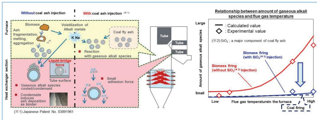
**Figure 2** Ash deposition mechanism and effect of ash deposition prevention by coal ash introduction
