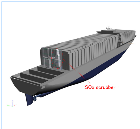
Figure 6 Conceptual image of scrubber located on board large container ship
