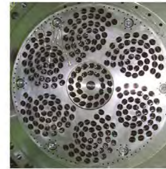
Figure 5 Multi-cluster combustor (under development)
