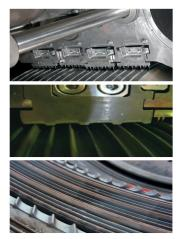
Mitsubishi Power Europe offers Active Clearance Control for shaft sealing systems to increase the sealing performance and improve efficiency of the unit. These modifications are simple and quick to apply to the unit and will reduce maintenance costs.
